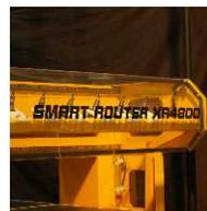
□ **Enclosed safety screen** protects operator from safety-critical areas of the machine. Provides for a safe working environment.
