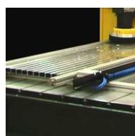
□ **Extrusion clamping system**
