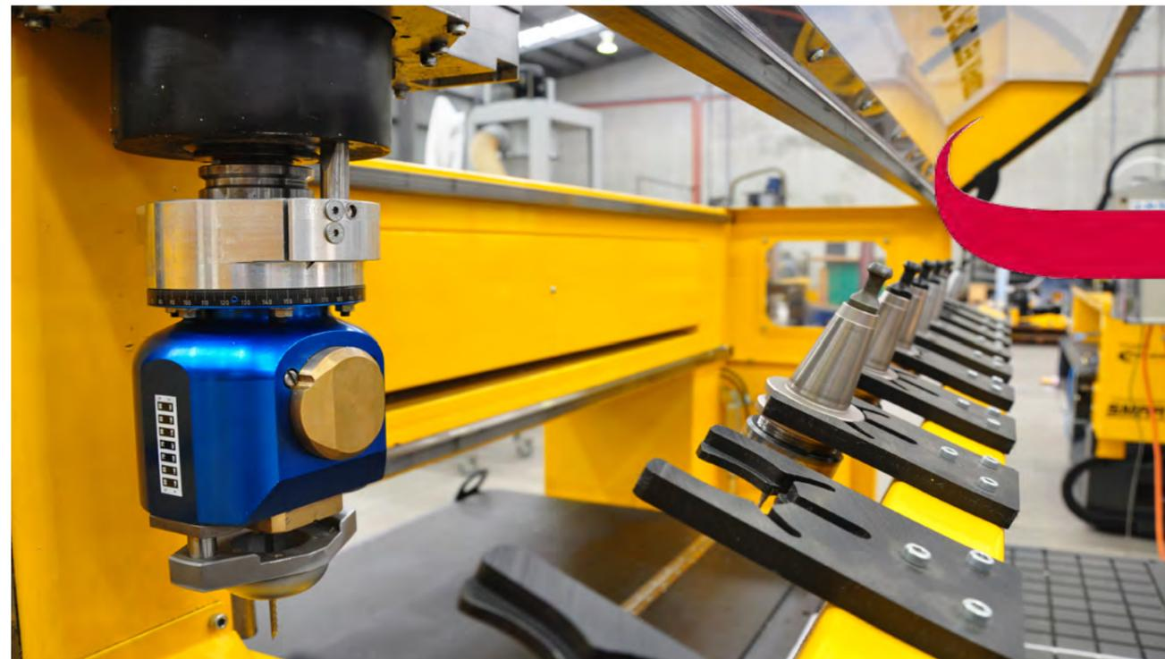
The gantry-mounted covered automated toolchanger turns creasing, variable-angle cutting, V-grooving and routing of insulated duct board into one efficient fully automated process.
