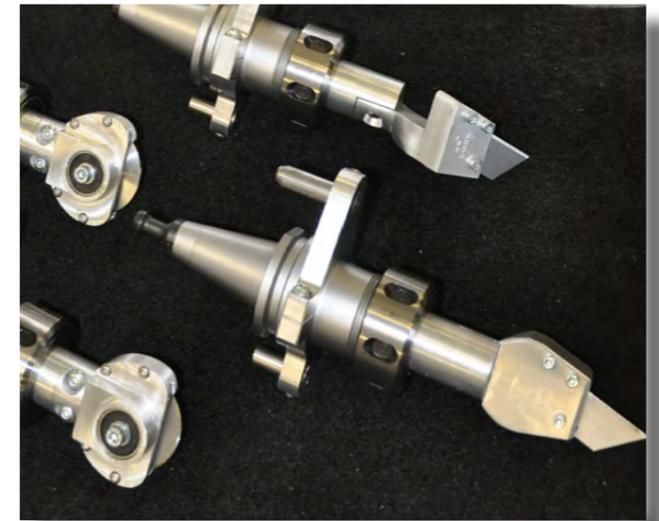
ART can help you by choosing the best tools for your material. With specialised V-Cutters to suit most material thicknesses and router bits to match so that you get the finished result, how you want it, time after time.
