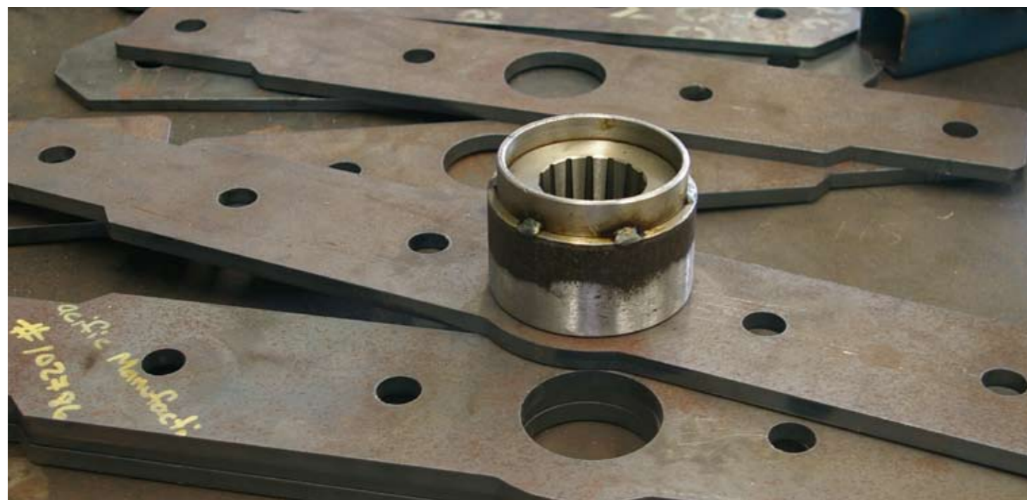
The CNC plasma cutter provides Pacific Manufacturing with the ability to cut the beams and blades from spring steel in-house. Eliminating outsourcing has provided the company with control over all production processes.
