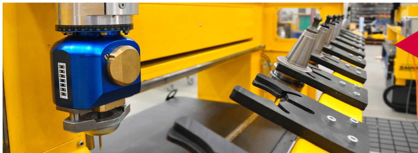
The gantry-mounted covered automated toolchanger turns creasing, variable-angle cutting, V-grooving and routing of insulated duct board into one efficient fully automated process.
